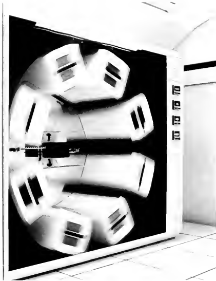
This mockup of a 1.8-meter centrifuge is undergoing tests at NASA's Marshall Space Flight Center. The centrifuge was designed at Ames Research Center for use on the Space Station.
